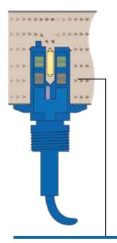
The robust Cambridge Viscosity oscillating piston system can measure a wide range of samples, including asphalt, lubrication oils, and heavy fuel oils, as well as handle any process upsets without damage to the system.
